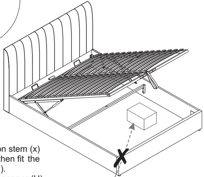
Slide gas-lift piston stem (x) onto the axle (y) then fit the flange lock-nut (F). Tighten nut with spanner (H) - do not over-tighten.
